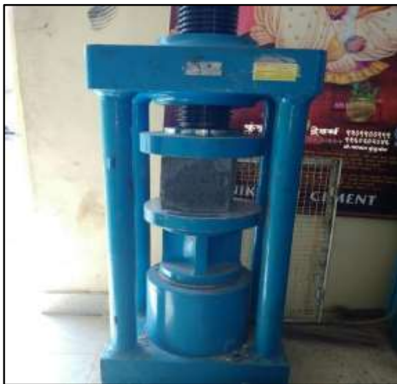
Fig 1. Compressive strength test
