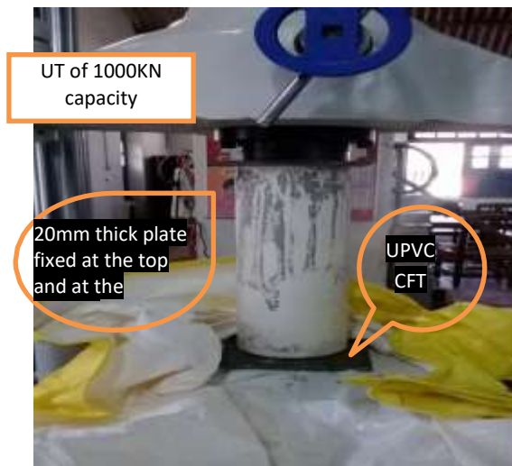
Fig. 6. Typical arrangement for loading using UTM
