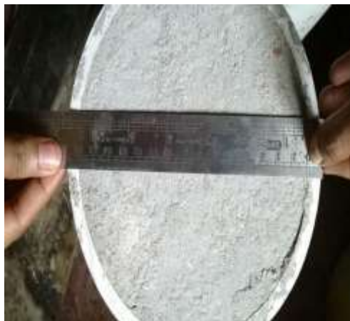
Fig 8: Increase in diameter (After testing)
