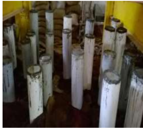
Fig.5. Water Curing by Ponding at the Top and Gunny Bags at the Bottom of Specimen
