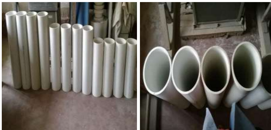
Fig 3: ASTM-D 1785 UPVC tubes of length 500
