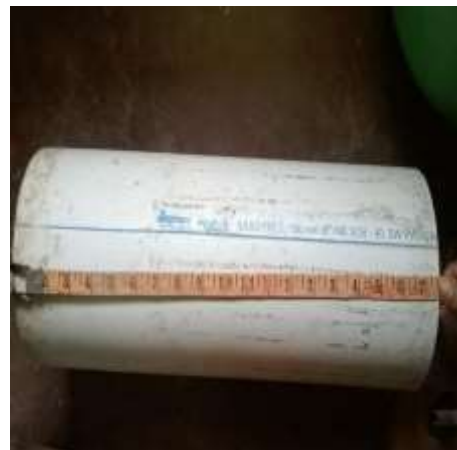
Fig 9: Decrease in length (After testing)
