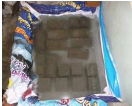
Figure 3. Curing of concrete
